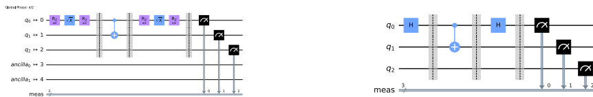
(a) A quantum circuit transpiled for real quantum hardware. In this case for the “ibmq_Lima”. (b) The same quantum circuit as in (a) transpiled for the “ibmq_qasm_simulator”.
