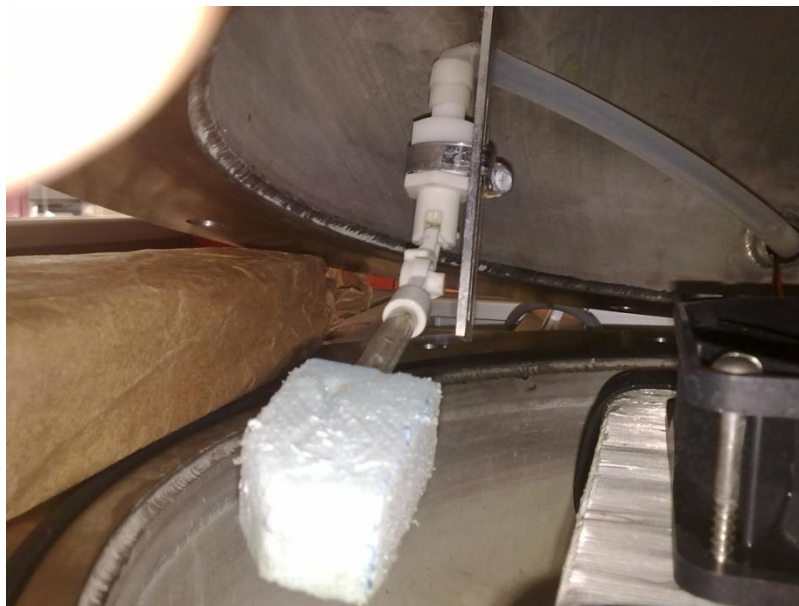
Figure 5.5 Water level valve
