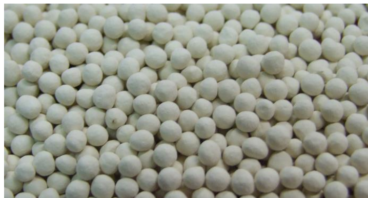
Figure 2.7 Köstrolith NaMSX spheres [Source: Fraunhofer IGB]
