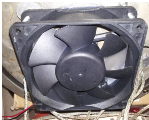
Figure 5.8: Fan used inside the reactor
