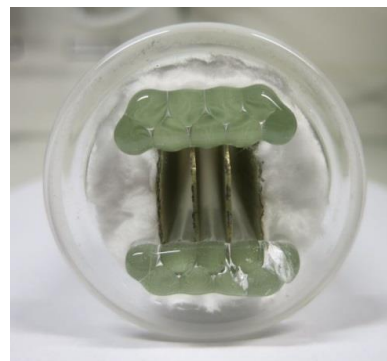
Figure 3-4: Plate catalyst installed in a catalyst holder
