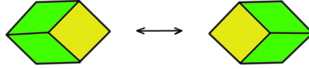
Figure 20: The elementary flip ('Simpleton') of the Ammann-Beenker tiling, or any square-rhombus tiling. Only one point in the center of the hexagon flips. (page 474 in [21])
