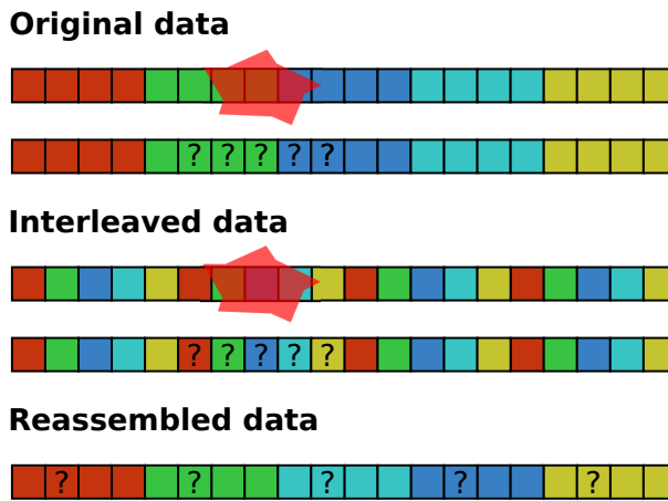
Figure 2.6: SEEs in memory with and without bit interleaving.
