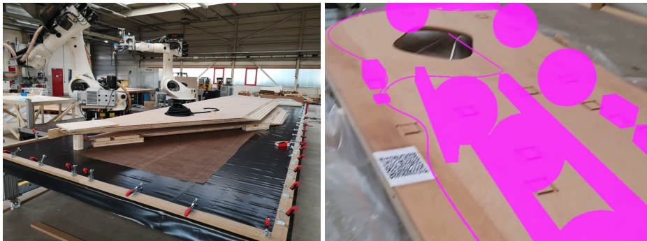
Figure 6.9: Lower ceiling timber panel (panel C) placed in the working environment at the laboratory (left) and lower ceiling timber panel (panel A) from the perspective of a worker, using the HoloLens and the AR system (with the different Unity objects and the fixed marker) (right).
