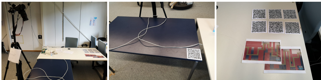
Figure 6.1: Simulated working environment for the user study, consisting of tabletop, cable, image target and digital camera.
