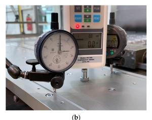
**Figure 14.** Setups of the force-dependent displacement measurements. (a) Testing of individual winding pins; (b) Testing of the whole assembled component (CFW structure located below the base plate).
