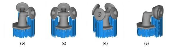
**Figure 7.** Support structure (blue) needed for the LPBF fabrication process. (**a**) Single-arm winding pin; (**b**) 2-arm winding pin; (**c**) 3-arm winding pin; (**d**) 4-arm winding pin; (**e**) Single-arm winding pin with secondary mounting point.
