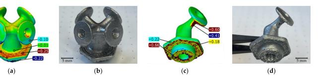
**Figure 6.** Computer tomography scans of the winding pins. Red areas represent oversized geometry, while blue represent undersized geometry in comparison to the target geometry. (a) CT-scan of the 4-arm winding pin, scale range from -0.2 mm to +0.2 mm; (b) Photo of the 4-arm winding pin; (c) CT-scan of the single-arm winding pin, scale range from -0.3 mm to +0.2 mm; (d) Photo of the single-arm winding pin.
