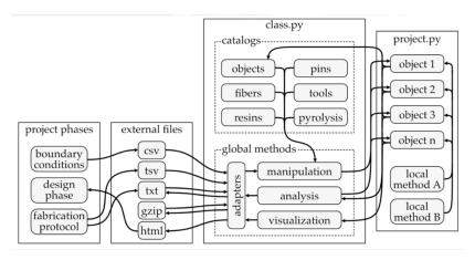
Figure 3. Domains of the CFW design and management tool. Multiple project files are possible.
