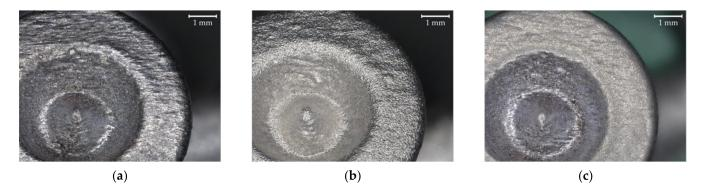
**Figure 8.** Light microscopic images of the disk area of a 4-arm winding pin. (**a**) Untreated surface; (**b**) Sandblasted surface; (**c**) Surface after barrel tumbling, area around the measuring tip is almost unaffected.
