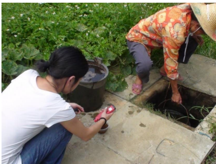
Figure 4-9 On-site pH value and temperature measurement
