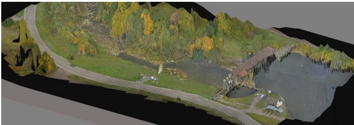
Fig. 84: Survey of the Murgtalsperre Kirschbaumwasen by an UAS in 2013 and a subsequent analysis with SfM (photo courtesy: I AM HYDRO).
