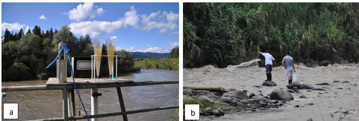
Fig. 56: (a) monitoring of the downstream suspended sediment concentrations during the flushing of the Fischeing reservoir, Austria, in 2012; (b) ecological monitoring downstream of the Peñas Blancas reservoir during flushing with partial drawdown in 2013.
