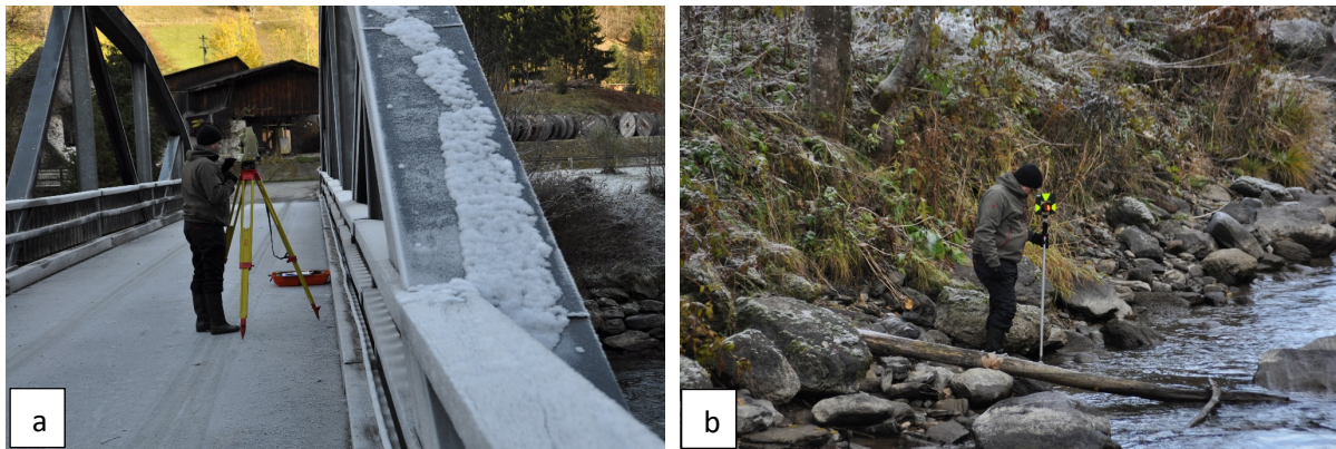
Fig. 82: Terrestrial survey along the Bodendorf reservoir, Austria, in 2010 (a) total station located at a fixed point on a bridge; (b) rover for taking points along the shore of the reservoir.
