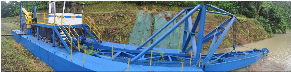
Fig. 51: Cutter suction dredge, installed at the Peñas Blancas reservoir in Costa Rica.
