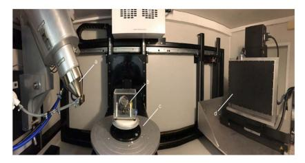
**Figure 8.** Measurement setup in CT: (**a**) X-Ray tube; (**b**) object to be scanned; (**c**) rotation table; and (**d**) flat panel detector.
