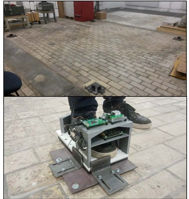
FIGURE 9. Test track (upper picture) and test shoe (lower picture).
