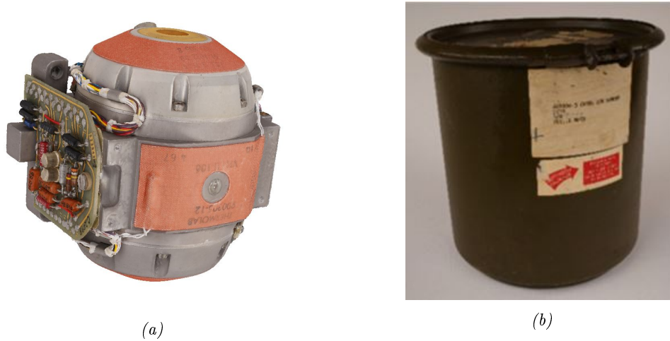
Figure 7.4: The Gyro G200 of the LN3 Inertial Platform: (a) Gyro G200; (b) G200 transportation box.
