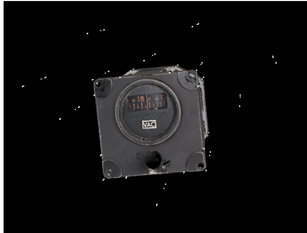
Figure 5.18: Virtual control points of photogrammetric model.
