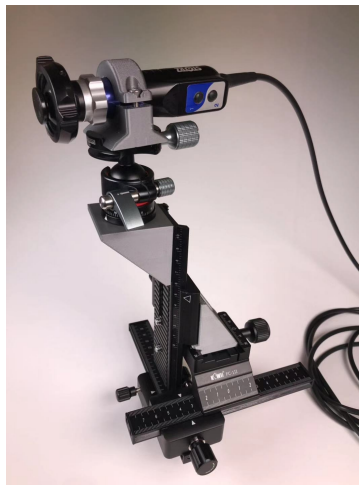
Figure 3.4: Self-designed endoscope imaging setup.
