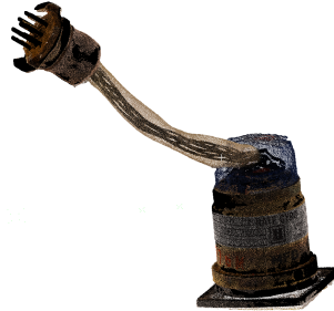
Figure 5.8: Aligned photogrammetric and CT surface point clouds.
