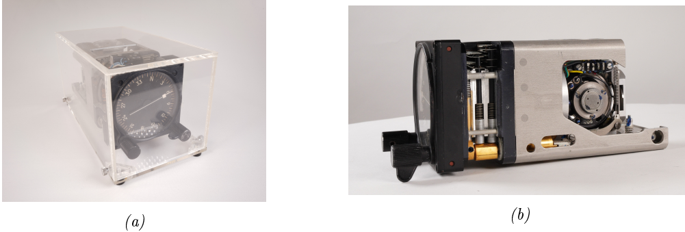
Figure 7.6: Directional gyro KK13-09: (a) general view; (b) side view without the caging device.
