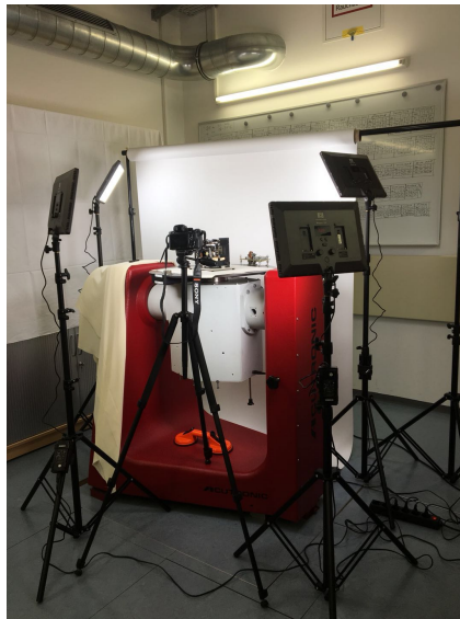
Figure 4.4: Photogrammetry turn-table setup.
