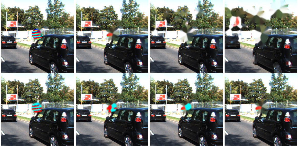
Figure 3.7: Visualization of the influence of the filtering threshold t and the scaling factor s on a patch and its environment. The top row displays decreasing values of the filtering threshold t \in \{0.3, 0.25, 0.2, 0.15\} with a fixed smoothing factor s = 10 . The bottom row illustrates increasing values of the scaling factor s \in \{2.5, 7.5, 20, 40\} with fixed filtering threshold t = 25 .
