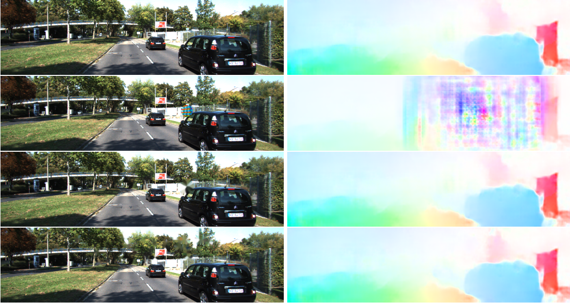
Figure 3.8: Visualization of the effect of ILP. The first column displays the first image of the image pair that served as an input to FlowNetC. The second column depicts the resulting optical flow prediction for four modalities. The modalities from top to bottom are: unattacked flow estimation without ILP pre-processing, attacked flow without ILP pre-processing, attacked flow with ILP pre-processing, unattacked flow with ILP pre-processing. The used parameter configuration is k = 16 , o = 8 , t = 0.25 , s = 10 .
