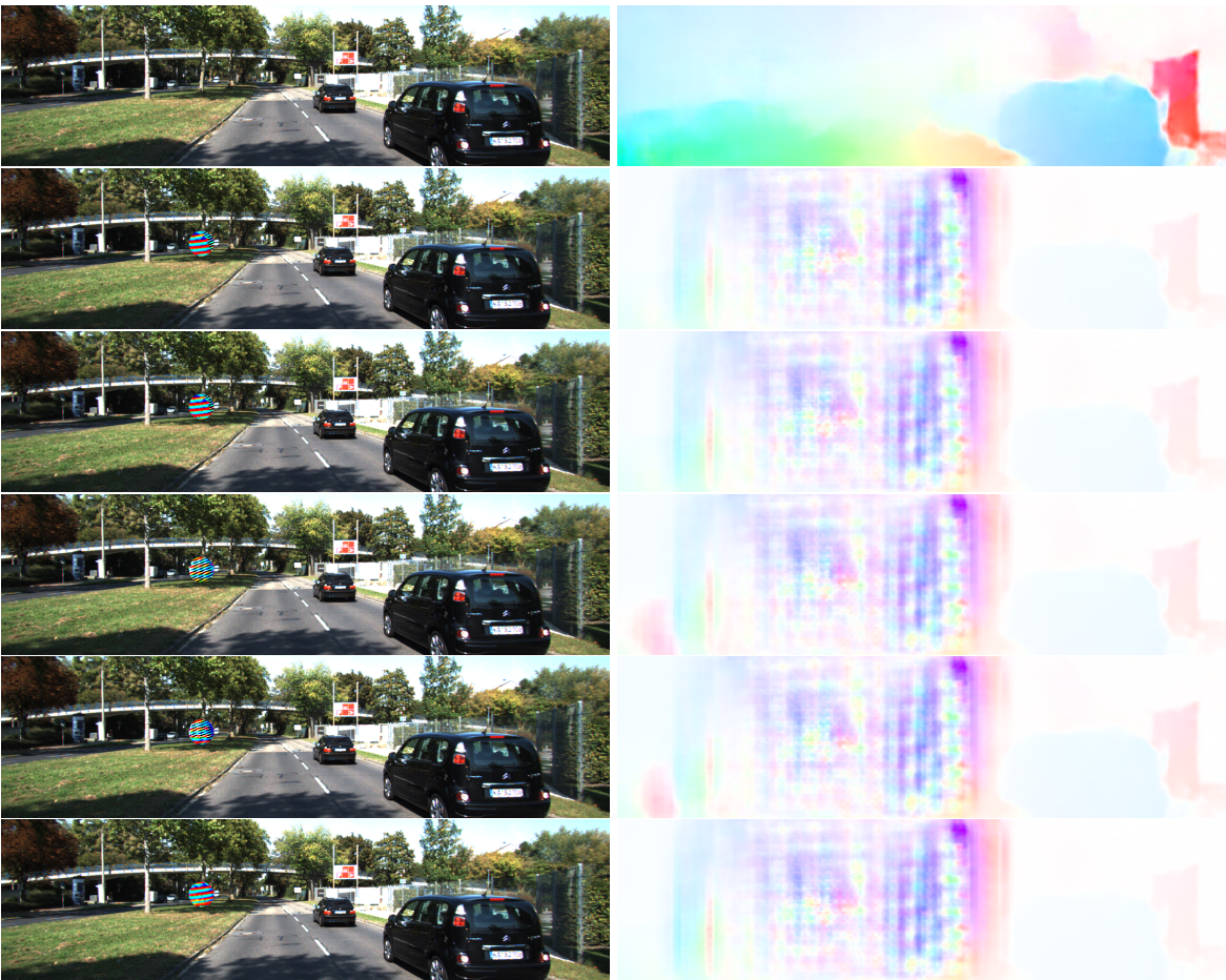
Figure 4.4: Influence of our adversarial patches trained with Algorithm 4.1 on the FlowNetC prediction result. The first row visualizes an unattacked input image together with the flow field estimation. The following rows present the results for images that are attacked by our patches of Run 1 to Run 5.
