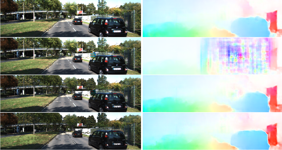
Figure 3.4: Visualization of the effect of LGS. The first column displays the first image of the image pair that served as an input to FlowNetC. The second column depicts the resulting optical flow prediction for four modalities. The modalities from top to bottom are: unattacked flow estimation without pre-processing, attacked flow without LGS pre-processing, attacked flow with LGS pre-processing, unattacked flow with LGS pre-processing. The used parameter configuration is k = 15, o = 5, t = 0.1, s = 2.3 .
