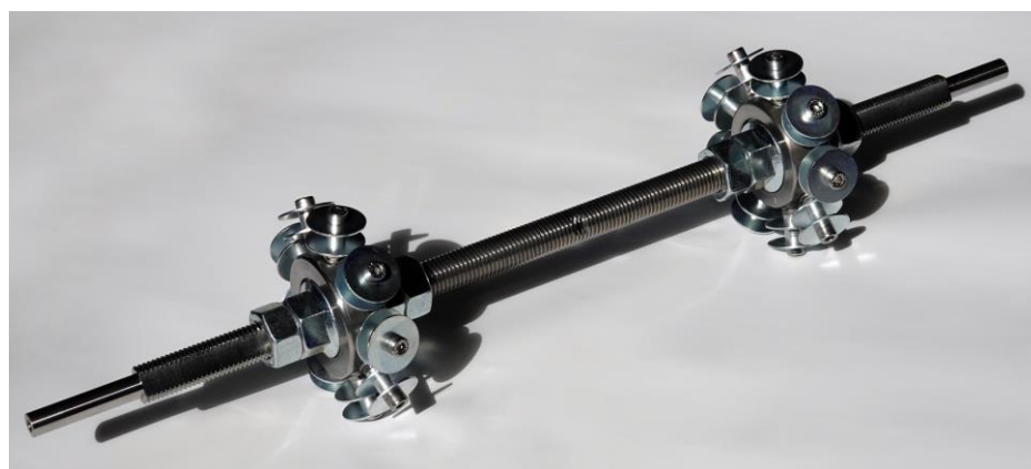
Figure 8. Winding fixture for the generic cylindrical samples equipped with medium size winding pins.
