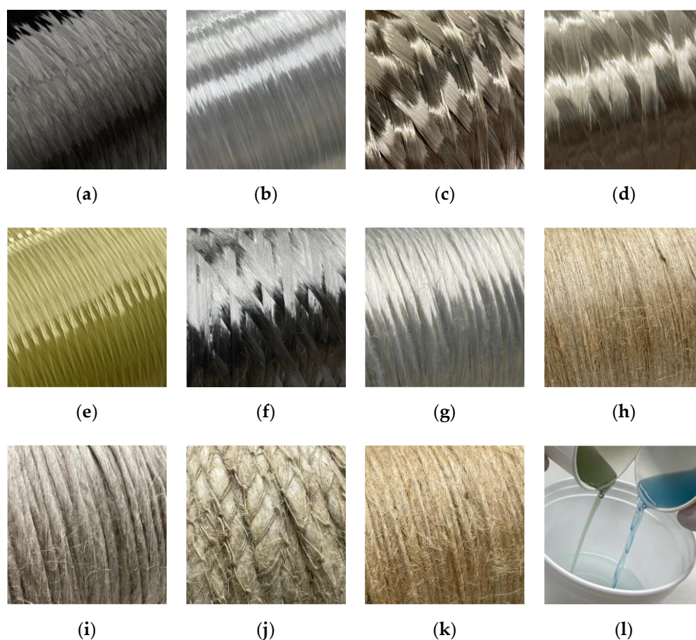
Figure 2. Material selection for this study: (a) carbon; (b) glass; (c) basalt type 1; (d) basalt type 2; (e) aramid; (f) stainless steel; (g) viscose; (h) flax tape; (i) flax yarn; (j) hemp (crocheted card sliver); (k) jute; (l) epoxy resin.
