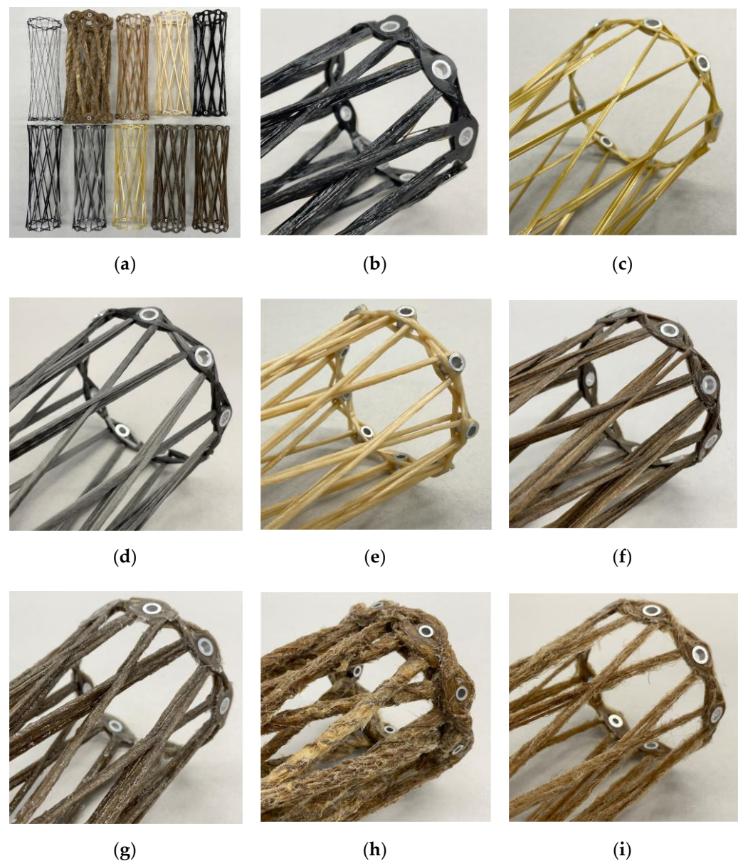
Figure 9. Selection of some of the produced generic cylindrical samples, from left to right and top to bottom: 1 \times 6k carbon, hemp, jute, viscose, basalt type 1, 3 \times 24K carbon, stainless steel, aramid, flax yarn, and flax tape. (a) Size comparison overview; (b) basalt; (c) aramid; (d) stainless steel; (e) viscose; (f) flax tape; (g) flax yarn; (h) hemp; (i) jute.
