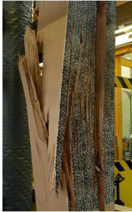
Figure 3.8. Combined tensile and transverse tension/shear failure at midspan of column S20.
