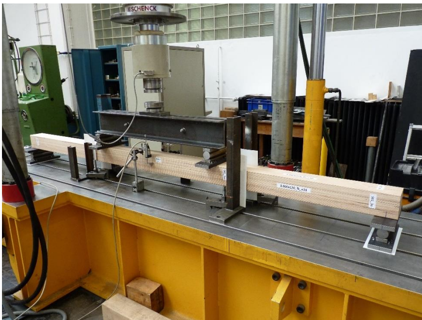
Figure 3.1. Elastic 4-point bending test with length x width x height = 2500 x 200 x 200 mm 3 .
