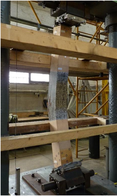
Figure 3.7. Column S22 after failure; test specimen “jumped” out of the tilting bearings when failure occurred.
