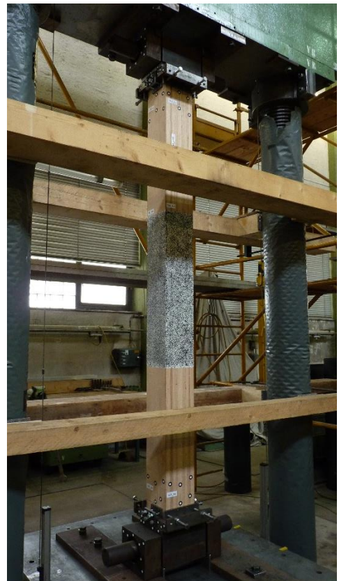
Figure 1.1. Buckling test of a beech LVL column with length x width x height = 2500 x 200 x 200 mm.
