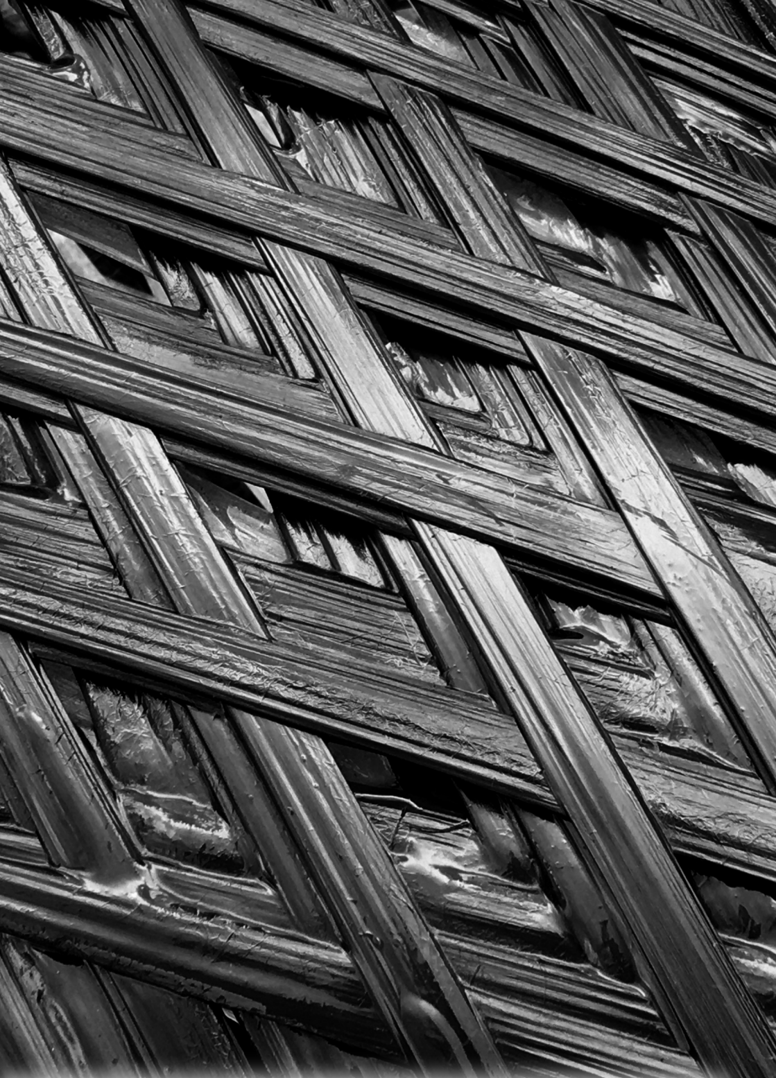
Lattice carbon-fiber reinforcement pattern of a fiber pavilion component showing the layerwise fiber deposition process.
