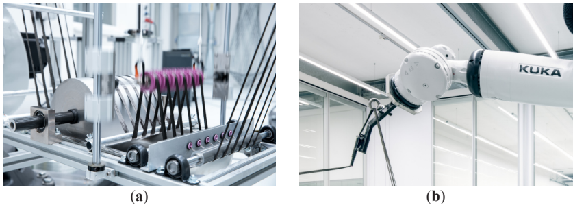
Figure 2.3 State-of-the-art CFW equipment. (a) drum resin bath with passive tension control and fibers traveling from left to right, (b) winding head with fibers traveling from bottom to left. © ICD/ITKE University of Stuttgart.
