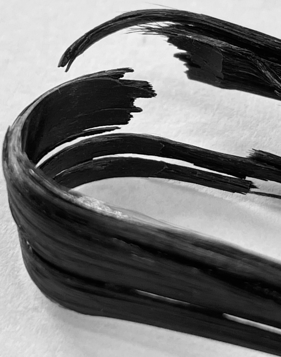
Loop specimen after failure exhibiting fiber fracture, delamination, and detachment from the sleeve.
