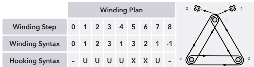
Figure 2.1 Example of a winding plan. Winding anchors (1, 2, 3), fixation points (0, -1), placement direction of the fiber (arrows), cut-off segments (dotted line), hooking steps with self-overlapping (X) and without (U). This illustration ignores the order of layers.
