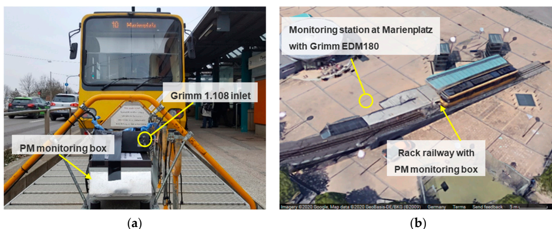
Figure 4. (a) The placement of aerosol spectrometer Grimm 1.108 along with the sensor-monitoring box, (b) The location of aerosol spectrometer Grimm EDM180 installed in the monitoring station at Marienplatz.
