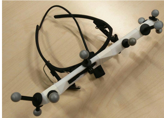
Figure 7.3: Eye-tracker with an attachment for placing additional motion capture markers.
