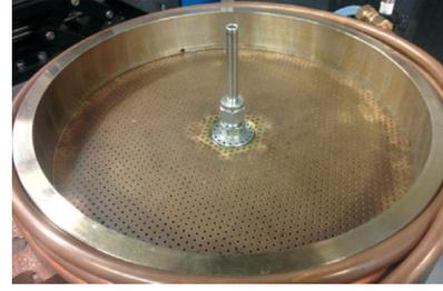
Fig. 1. Modified version of the Cabra burner.
