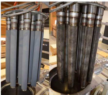
Fig. 8 Metal mesh filter before and after cleaning
