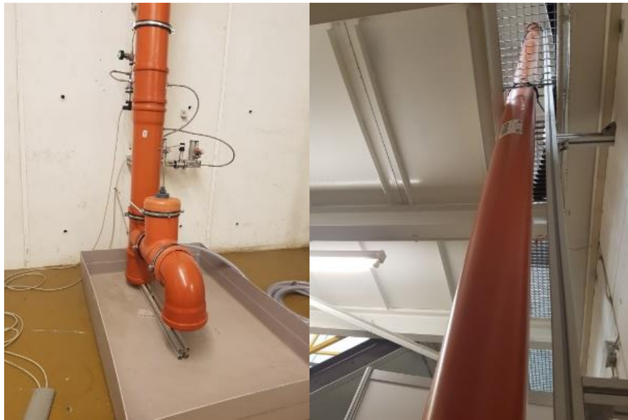
Figure 4.3 Measurement set-up in IKE laboratory for the modified falling head method. Left: The lower part of the set-up with instrumentation, sample placement area and opening valve. Right: View from below to the entire height of the set-up.
