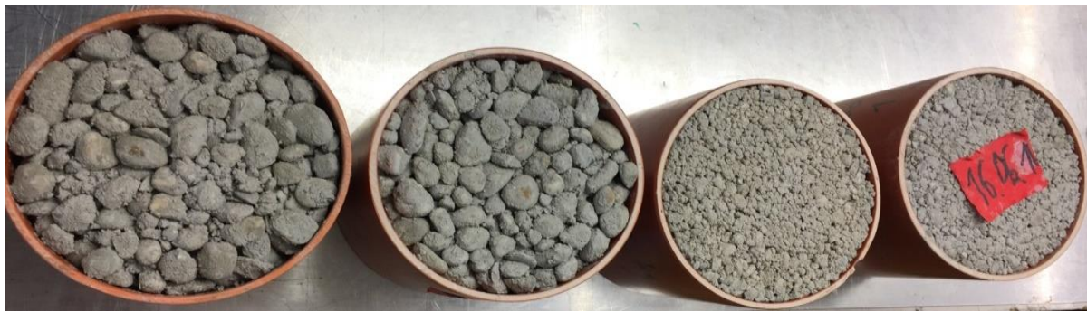
Figure 4.1 Porous concrete samples from KIT. Samples left to right: C1, C2, F1, and F2.
