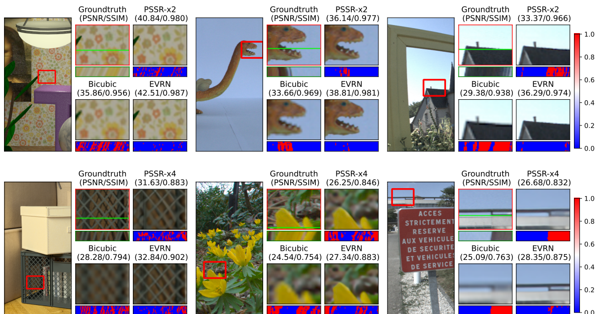
Figure 5.8: Comparison of two stages in reconstruction of spatially high resolution LF. The SAI at \theta = (4, 4) is visualized together with its zoom-in region marked by a red rectangle. For each approach, an EPI at horizontal line marked in green is extracted and compared to the EPI of Groundtruth. The first row, from left to right: \times 2 results of synthetic scene mona [14] and real-world scenes Ankylosaurus_&_Diplodocus_1 , Framed [18]. The second row, from left to right: \times 4 results of synthetic scene boxes [4] and real-world scenes Flowers , Sign [18].
