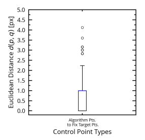
**Figure 7.** Euclidean distance between algorithm found control points and the fix grid control points for the dataset of 54,835 control points. The whisker lengths indicate 0% percentile to 99% percentile.
