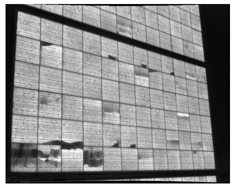
**Figure A3.** DaySy<sup>™</sup> electroluminescence (EL) image after distortion correction. Straight line structures in the PV module are represented by straight line structures in the image.
