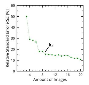
**Figure 4.** Relative Standard Error (RSE) of the distortion coefficient  $k_1$  for the parameter estimation in Figure 1 with respect to the number of images in the calibration dataset (f = 25 mm). The RSE decreases with the number of image planes used for the parameter estimation. In our dataset the error  $k_1$  becomes reliable with seven or more images for calibration as the RSE falls below 20%.
