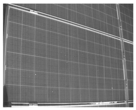
**Figure A2.** Original DaySy<sup>™</sup> photography image of Solarzentrum Stuttgart GmbH affected by barrel lens distortion. Straight line structures in the PV module are represented by curved line structures in the image.
