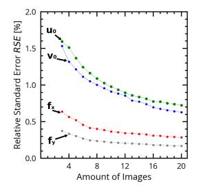
**Figure 3.** Relative Standard Error (RSE) of the focal length camera parameters ( $f_x$ ,  $f_y$ ) and the principal point camera parameter ( $u_0$ ,  $v_0$ ) for the parameter estimation in Figure 1 with respect to the number of images in the calibration dataset (f = 25 mm). The RSE decreases with the amount of image planes used for the parameter estimation. All RSEs show a small value and therefore a good estimation accuracy
