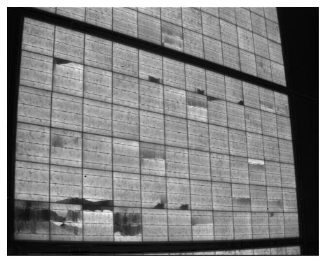
**Figure A1.** Original DaySy<sup>™</sup> electroluminescence (EL) image of Solarzentrum Stuttgart GmbH affected by barrel lens distortion. Straight line structures in the PV module are represented by curved line structures in the image.
