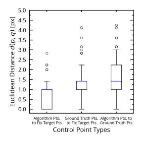
**Figure 8.** Euclidean distance between the control point types for the 40 EL ground truth EL images (2200 control points). The whisker lengths indicate 0% percentile to 99% percentile.
