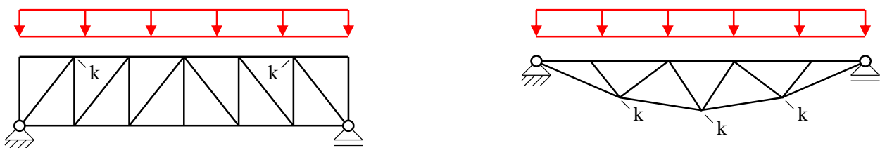
Fig. 6.1: Examples for kink points k in tension and compression members of trusses [70]
