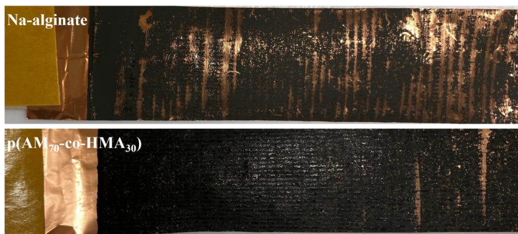
Figure S6: Optical images of the Si coatings prepared with Na-alginate (upper panel) and p(AM 70 -co-HMA 30 ) (lower panel) after conducting a 180° peel test.
