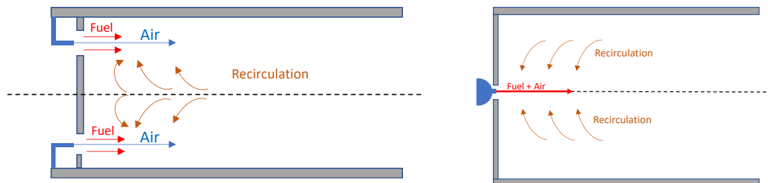
Figure 26 Comparison of the recirculation principle for multi-nozzle (left) and single-nozzle (right) design
