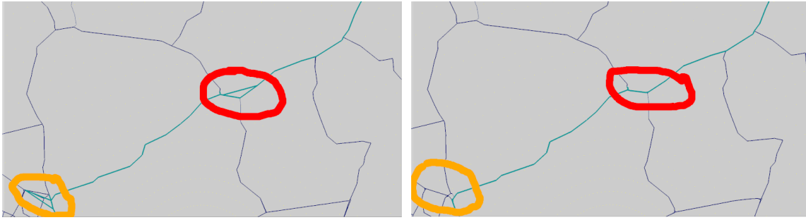
Figure 8.10.: Topological inconsistencies of complex network parts (left) vs topologically correct representation (right).
