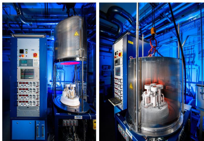
Figure 34 Cell test bench for high temperature electrochemical characterization of solid oxide cells with 4 cell positions and 4 independent electrical loads.
