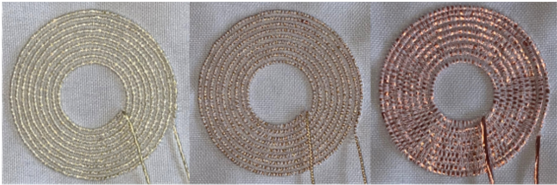
Figure 4. Embroidered coils with a diameter of 40 mm (from left to right) 40E12 ELITEX, 40U12 wrapping yarn, 40L12 copper wire.
