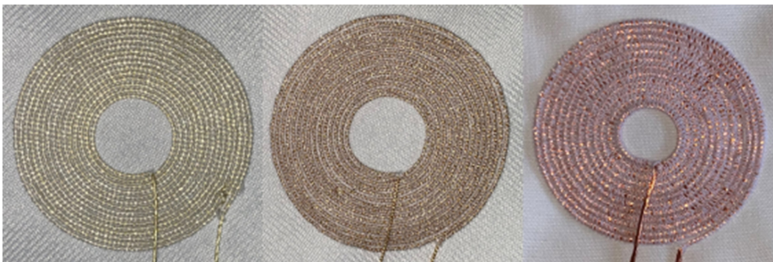
Figure 3. Embroidered coils with a diameter of 50 mm (from left to right) 50E12 ELITEX, 50U12 wrapping yarn, 50L12 copper wire.
