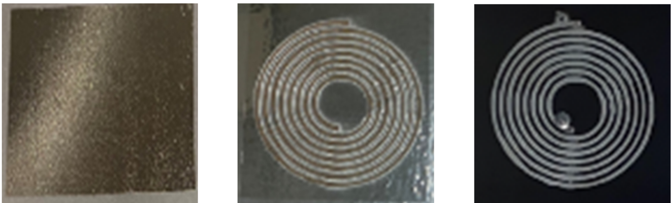
Figure 6. Printed coils according to the Qi standard: Primer (left), printing stencil (middle) and printed coils (right).
