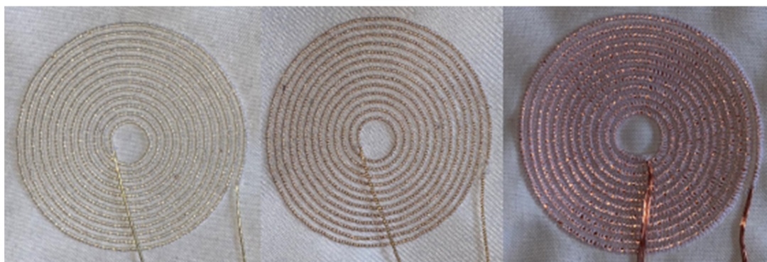
Figure 2. Embroidered coils with a diameter of 60 mm (from left to right) 60E12 ELITEX, 60U12 wrapping yarn, 60L12 copper wire.
