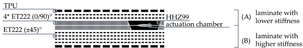
Figure 11. Schematic sketch of laminate set-up with stiffened flaps due to the substitution of HHZ99 by four layers ET222 (fiber orientation 0/90°) (HHZ99 layer on laminate side (A) with lower stiffness 5 cm wider than on laminate side (B) with higher stiffness).
