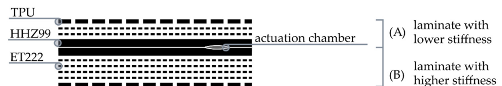
Figure 3. Schematic of an exemplary laminate set-up (TPU/ET222 4 /HHZ99 2 /ET222 2 /TPU), where ET222 is implemented with a fiber orientation of \pm 45^\circ .
