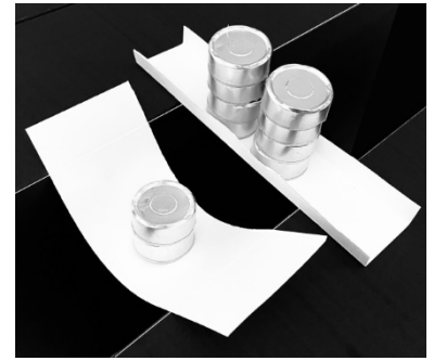
FIG. 2.42: A single, flat paper strip (left), and a single, channel-folded paper strip (right) demonstrate the influence of the cross-section on the bending stiffness of a system.
