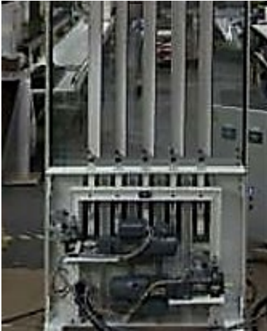
FIG. 1.21: Flectofin® demonstrator actuated by electric motors. (Photo by ITKE)
