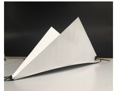
FIG. 3.81: Flectofold with inconspicuous, integrated pneumatic actuation in the curved folding lines.
