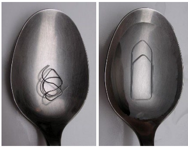
FIG. 2.7: Nitinol Memory Alloy paperclip in deformed state (left) and with restored shape due to heating (right). (Photos (left & right) by Petermaerki / CC BY-SA 3.0)
