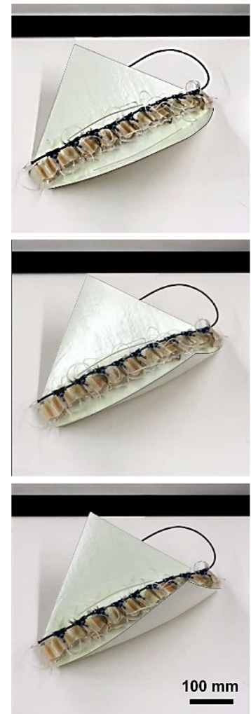
FIG. 3.21: Physical prototype of the single cell row actuator actuating the 2-dimensional compliant shading device Flectofold. With increasing pressure from top to bottom the midrib of the compliant shading system Flectofold bends further and thus causes the folding of the flaps. Adapted from (Mader et al. 2020b).
