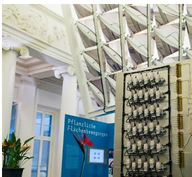
FIG. 4.1: Control panel of large-scale Flectofold demonstrator with 36 individual pneumatic actuators. (Photo by ITKE)
