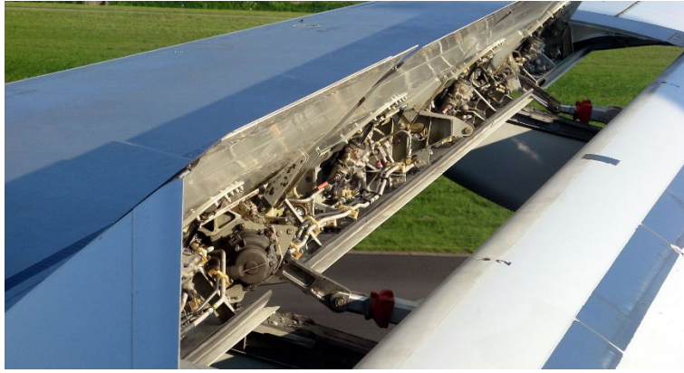
FIG. 1.3: Complex structure of the control surface of an airplane wing. (Photo by Annom / CC0)
