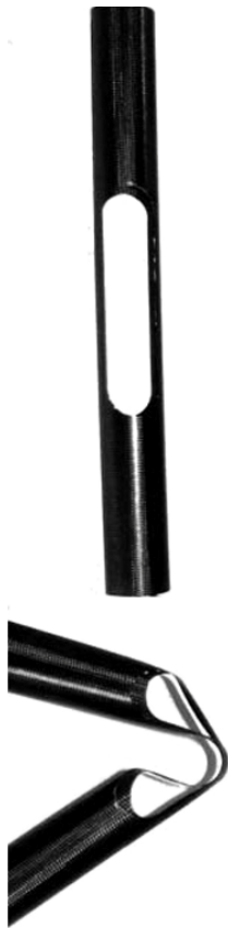
FIG. 1.10: Tape-spring hinge for deployable space structures fully deployed, partially folded. It is made from ultrathin two-ply plain-weave laminate of carbon-fiber reinforced plastic. Adapted from (Mallikarachchi and Pellegrino 2011).
