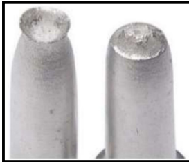
Figure 1.3: The so-called cup-cone failure occurs in ductile metals under uniaxial loading. The failure mode is named after the shape of the fracture surface. It originates from growth of micro voids in the metal. On the left a cup-cone failure from a tension test is shown. The right shows the numerical simulation results of such a tension test, see Chapter 4 or Miehe et al. 2016. Here the red color indicates the fracture surface.
