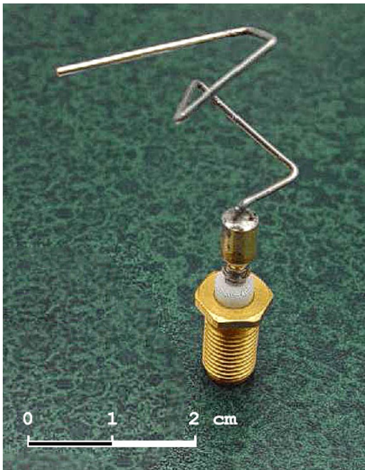
Fig. 5 NASA public domain picture of the St 5 X-band antenna, launched on a microsatellite as part of the Space Technology (ST5) mission in 2005 [48]. The evolved antenna meets the mission specification of a required, nearly uniform gain for a spinning satellite. NASA public domain picture of the St 5 X-band antenna, launched on a microsatellite as part of the Space Technology (ST5) mission in 2005 [48]. The evolved antenna meets the mission specification of a required, nearly uniform gain for a spinning satellite
