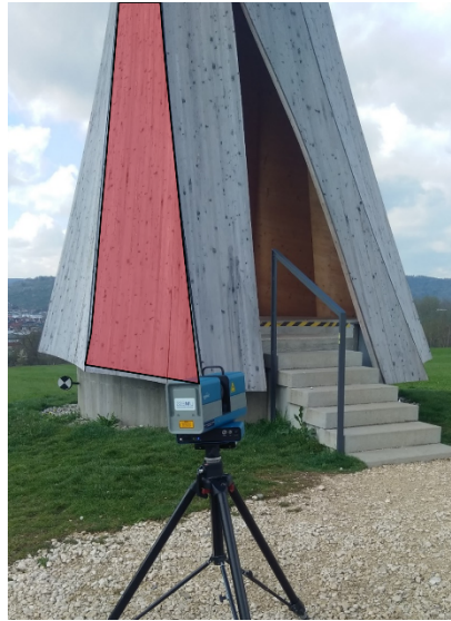
Figure 6.20 Selected surface of the tower façade, which is analyzed for deformations.
