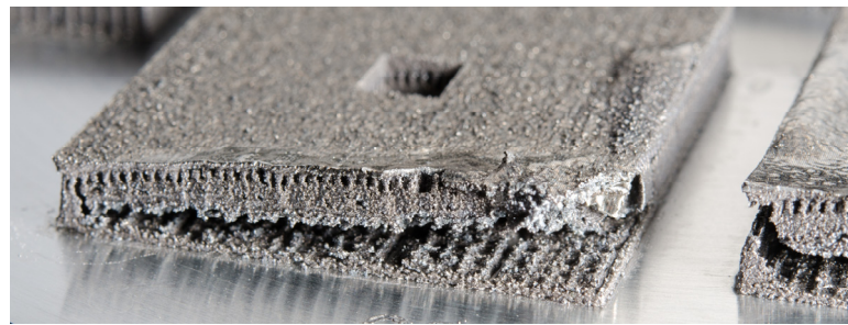
Figure 1. Distortions and delamination during manufacturing process leading to process failure.
