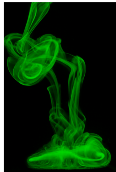
Fig. 15 Exemplary photograph (standard color DSLR camera) of a flow induced by dropping fluorescent liquid into water
