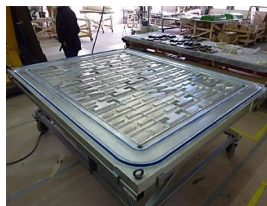
2-Mold before applying the fibre, resin and vacuum
