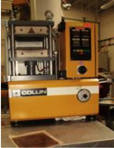
Figure C 1-9. Press machine used in thermal pressing of the discharge taken out of the batch mixer, to form the plate needed.
