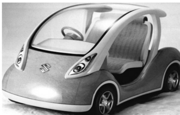
Figure B3-20. Concept of using banana mat fibre and epoxy resin by SUZUKI in the electric vehicle's body, (Krishnan, M.; Gruntechn Polymer Consultants, 2013)
