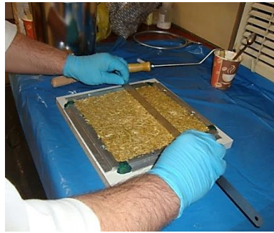
5-Checking the homogenous and full mixture distribution within the mold
