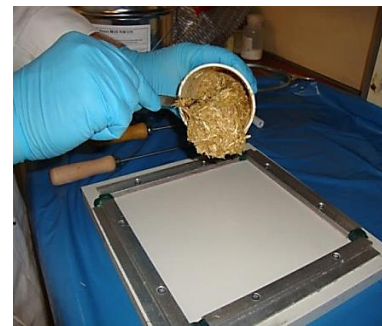
3-Pouring the mixture in the mold, after applying the suitable molding wax
