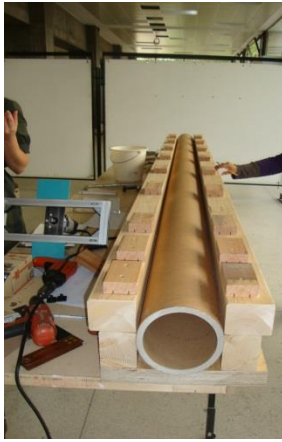
Fixing the cartoon columns in the wooden frame to guarantee fixation during the drilling process
