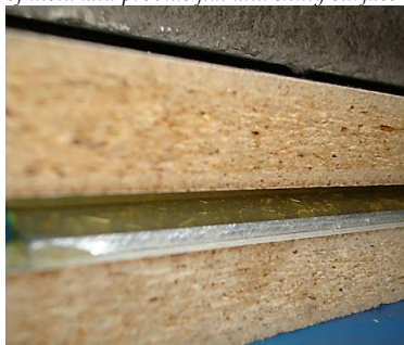
10-Excess resin is released out of the mold with the help of the frame openings
