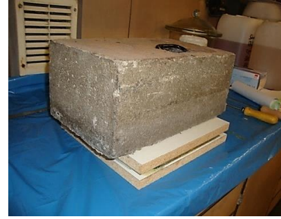
9-Providing excess load on the mold to provide enough pressure
