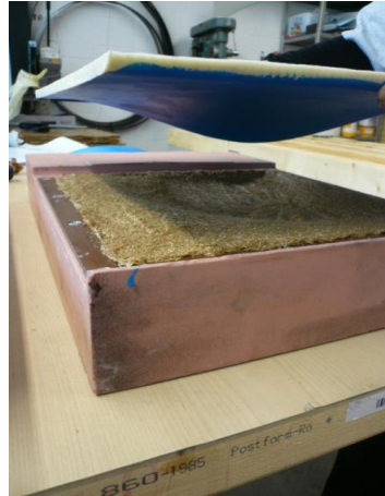
Covering the mixture within the positive mold-part
