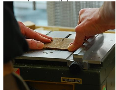
12-Cutting the test samples using a wood saw machine
