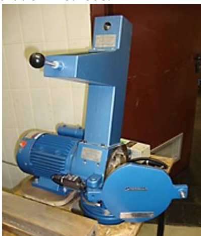
Figure C 1-3. Regular fibre chopping machines without dust absorbers
