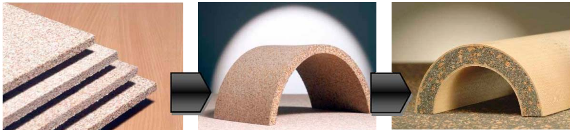
Figure D 1-8. Illustration of turning the elastic fibreboard Recoflex® from BSW Firma from a flat board to a 3D formed one through bending, then fixing the form through veneering, photo credit: (BSW BerleburgerSchaumstoffwerk GmbH, 2013).
