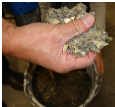
2- The mixture shouldn't be extra humid
