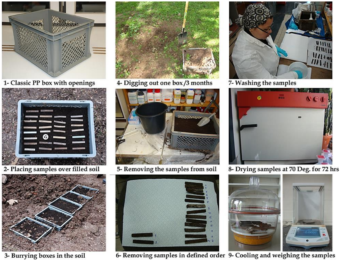
Figure C 1-21. Illustration of the soil burial biodegradability test scenario and control procedures
