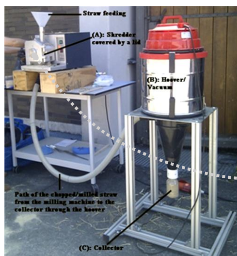
Figure C 1-5. Chopping machine provided from FRITSCH GmbH, where the 3 components are combined: shredder (A), Hoover- vacuum absorber (B) and collector (C) .
