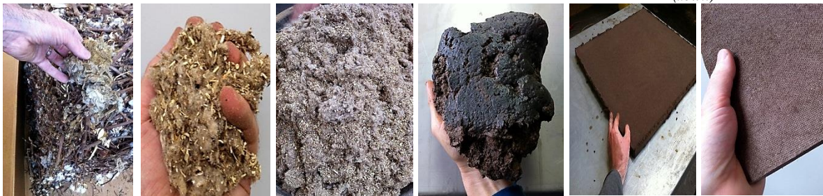
Cotton bush-the agricultural by-product after cotton harvesting, transferred into an insulating board using 'CORE' technology. Published after permission from R.Hurding- Zelfo Technology GmbH
