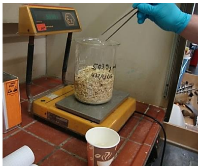
2-Weighing the straw with a high sensitive device with \pm 0.1 mg tolerance
