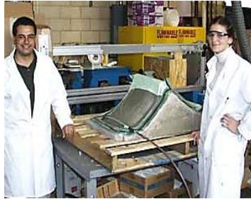
The manufacturing of the chair in process with room-temperature cured acrylated epoxidized soy oil (AESO), (Thompson, 2004)
