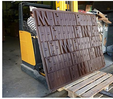
5-Final panel after vacuum molding process
