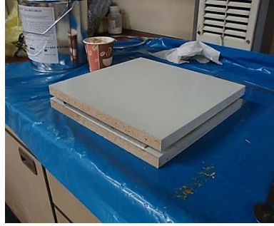
8-Covering the mold with the lid
