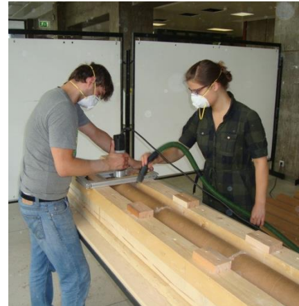
Drilling process taking place according to defined distances, to be ready for the dry fixation process through the wooden dove-tails
