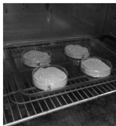
Figure C 1-2. Chopped rice straw samples dehydrated at 105°C for 24 hours
