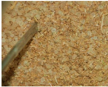
1-The RS-PLA were pre-mixed before dosing the mixture in the extruder
