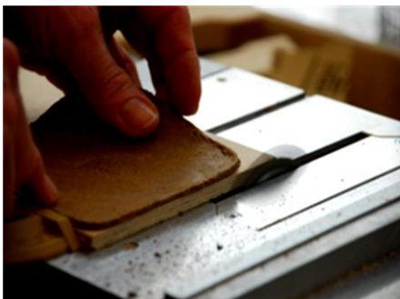
Figure C 1-11. Cutting process of the boards produced according to the sample dimensions defined
