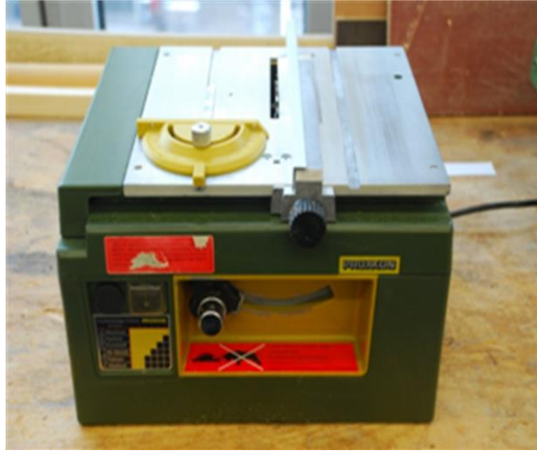
Figure C 1-10. The saw cutting machine applied in samples' preparation
