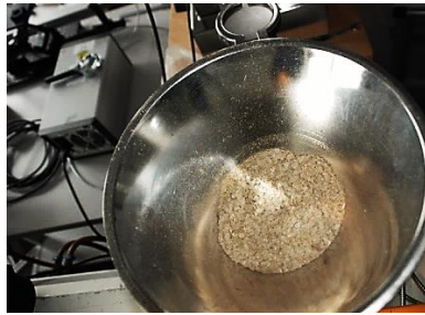
2-Applying the prepared mixture within the extruder
