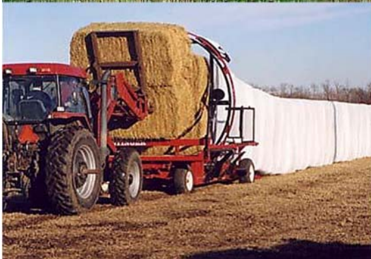
Figure B1- 8. Different baling systems (Huisman, et al., 2002). Up: square-bale individual wrapping, Down: Tube-wrapped system
