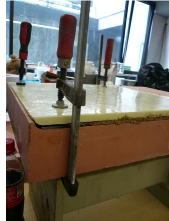
Casting the mixture in a closed molding process
