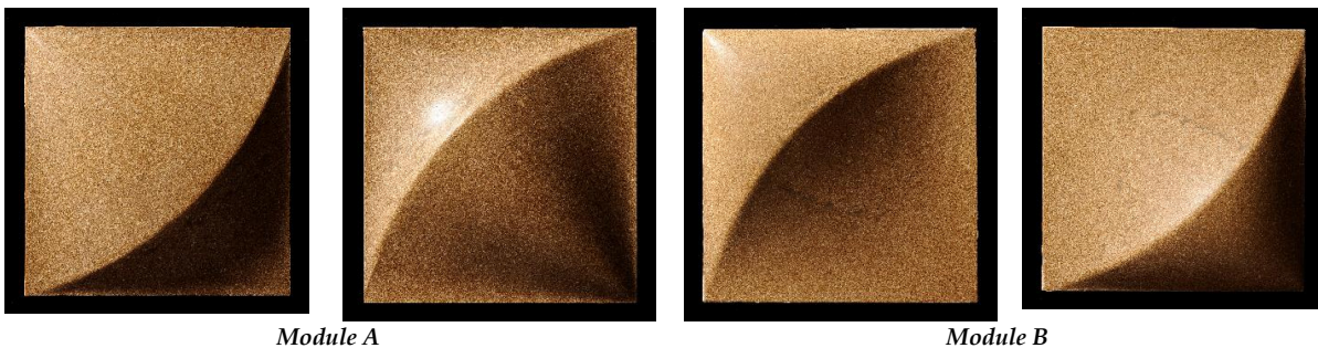
Figure D 3-4. Modules (A) and (B) settled in 2 opposite positions, to show the possible design variations, that was applied in the 3D-façade, applied in the 'Eco-Pavilion'. Photo credit: B.Milklausch
