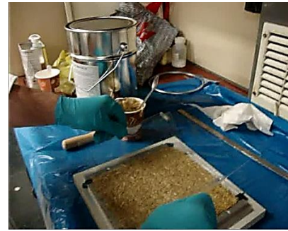
6-Applying the transparent foil on the mold to roll air bubbles out of mold
