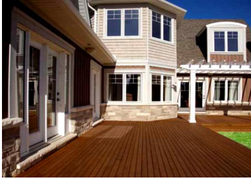
Figure B3-14. TerraDeck™ of recycled HDPE and straw, (Natures Composites TM- organic building products, 2011).
