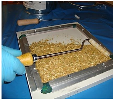
4-Spreading the mixture with a roller
