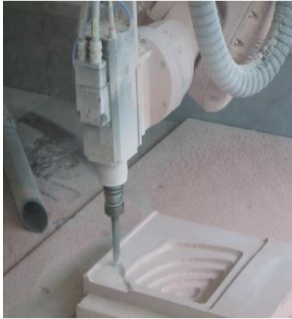
The robot-machine carving the negative casting mold, out of (PU 500) foam material.
