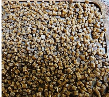
4-The RS-PLA pellets before being pressed in the heat-press machine
