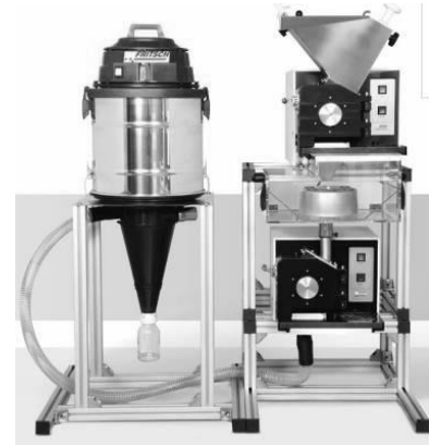
Figure B1-12. The chopping machine is integrated with the collector and dust absorber. (FRITSCH GmbH)
