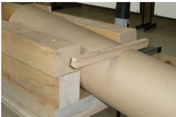
1-Experimenting the stabilization of the wooden connectors within the drilled slots in the cartoon pipes
