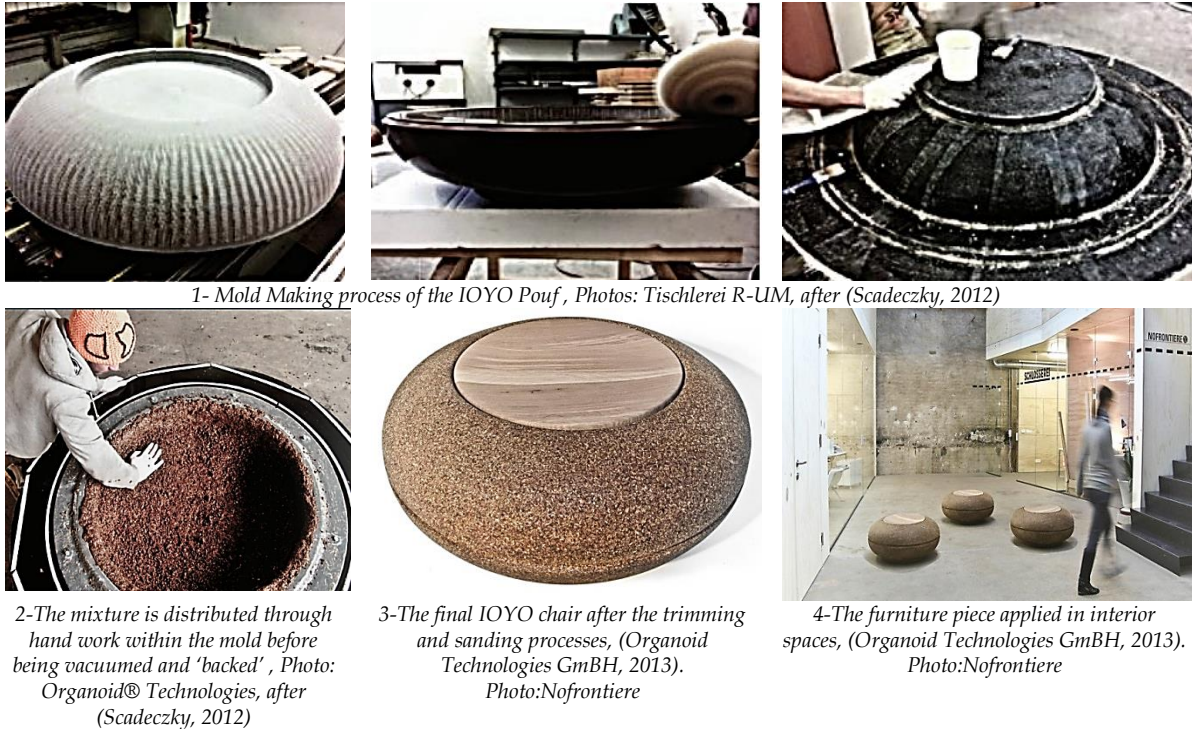
Figure B3-22. The manufacturing processes and application possibilities of a furniture model composed of a thermoset agro-fibres biocomposite, developed by Orngaid Technologies GmbH-Austria
