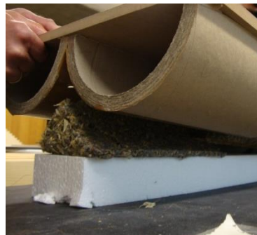
5- Releasing the molded insulation for de-hydration
