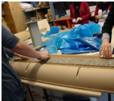
4- The molded insulation should be compact and dense
