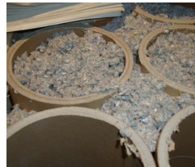
6- Possibility of filling the hollow columns with cellulose insulation for passive housing applications
