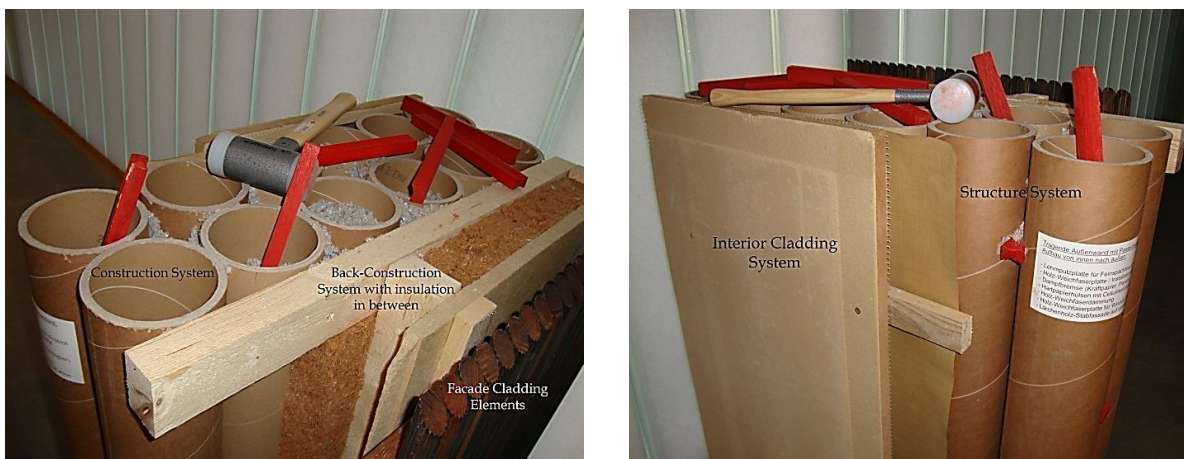
Simulation of the façade panels' fixation possibilities with the installed insulation within the back-construction
