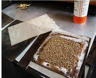
5-The pellets in the copper mold, covered by the Teflon® foils, before being pressed
