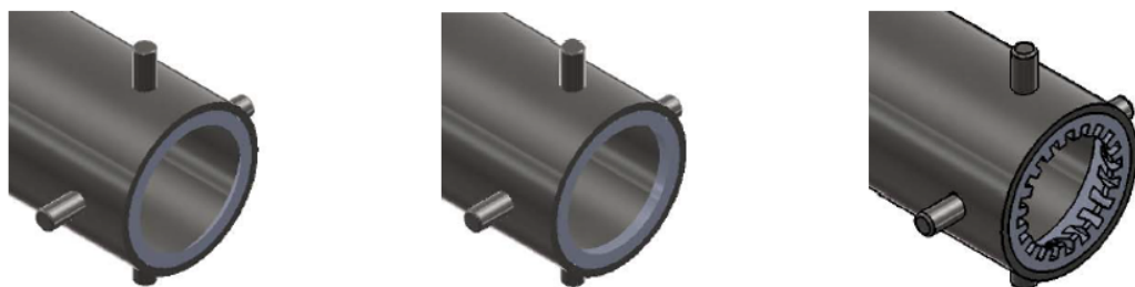
Figure 3.5: Primary air nozzle design, from left to right: Nozzle 1, Nozzle 2 and Nozzle 3
