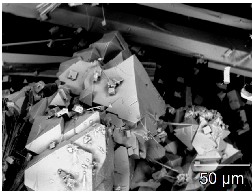
Figure 1. Electron micrograph of some crystals with the composition La_5Cl_3[SbO_3]_4 . The long rods visible at the upper edge of the image originate from a silicate by-product (apatite-type La_{4.667}O[SiO_4]_3 [17]).
