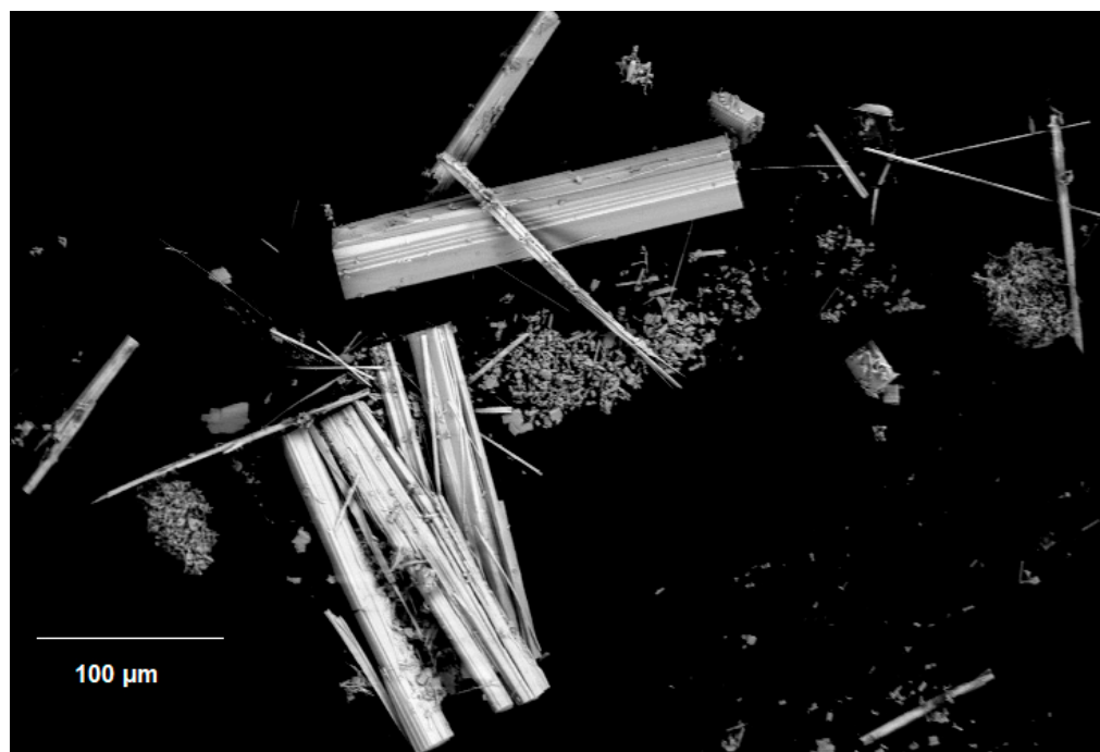
Figure 2. Electron-microscopic backscattering image of some acicular crystals of composition \text{La}_2\text{Sb}_{12}\text{O}_{19}\text{Br}_4 .
