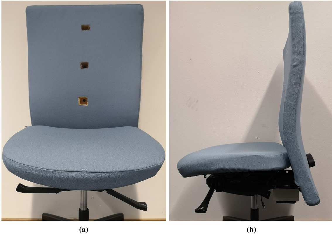
Figure 4.1: Our smart chair prototype shown from the front, where the Time of Flight (ToF) sensors can be seen (a), and from the side with the enclosure of the microcontroller and the power bank visible in the lower right corner (b).
