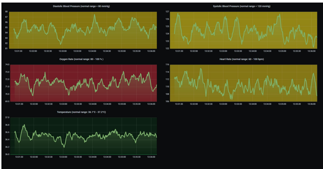
Figure 4.8: Grafana graphs when a few vitals are either critical or slightly above threshold. This is indicated by the colors of the background. Red shows that the vital is at its extreme limits and needs immediate attention. Yellow means that the readings are slightly above/below the normal range but not dangerous. Green shows that the vital is in its normal range and healthy
