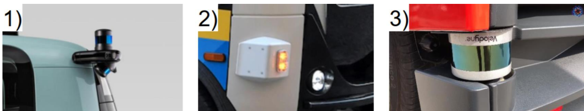
Figure 5: Integration of sensors at the macro level; 1) significant change to the body, own sensor carrier 2) moderate change, additional body element 3) no change to the outer contour
