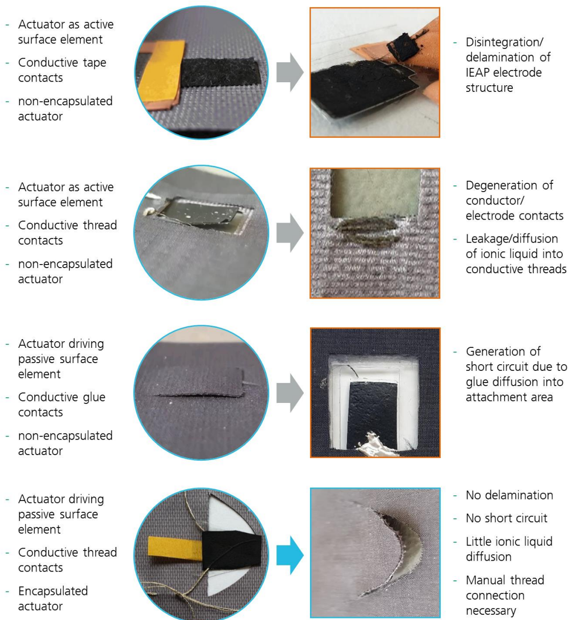
Figure 69 – Illustration examples of IEAP actuator/sensor integration. (Pictures: Nima Zahiri, IFF/BioMat 2019, edited by Raphael Neuhaus, IFF 2020)
