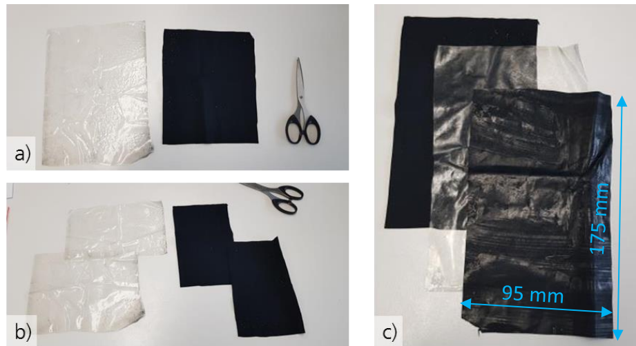
Figure 54 – Manual preparation of actuator layers for fusing-cutting approach
