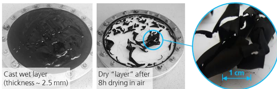
Figure 33 – Disassociation of dried MWCNT electrode layers into small curled-up pieces (pictures: Raphael Neuhaus, IFF)
