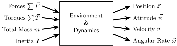
Figure 7.1: Inputs and Outputs of the Environment and Dynamics Simulation
