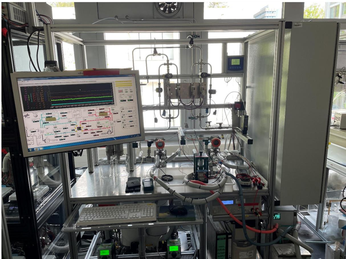
Figure 10. Testbench for standard PEM electrolysis cell operation with conventional BoP
