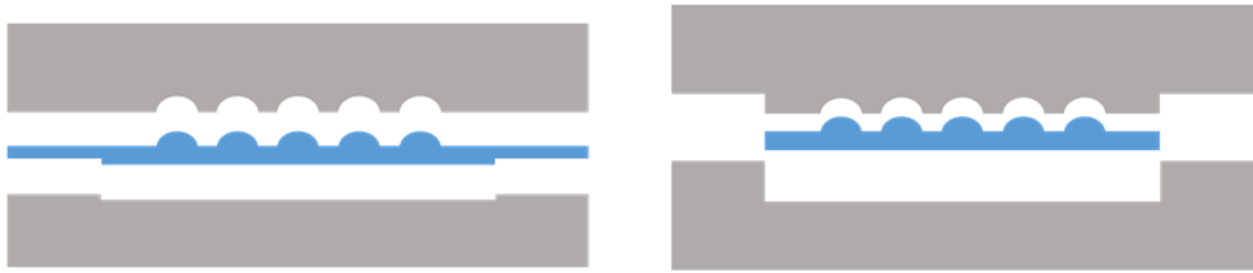
Figure 4-5: left: hot embossing; right: compression molding
