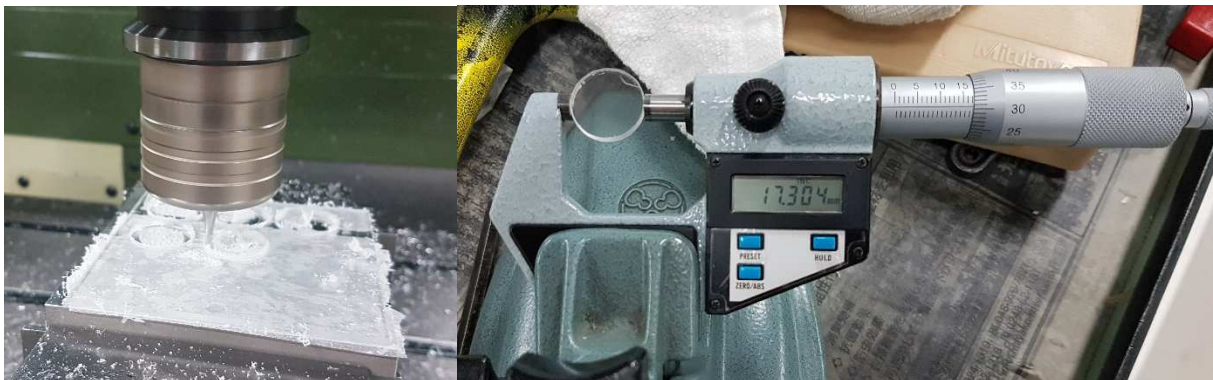
Figure 6-10: Preparation of cylindrical polycarbonate sheets; left: milling of samples; right: Diameter measurement using a micrometer
