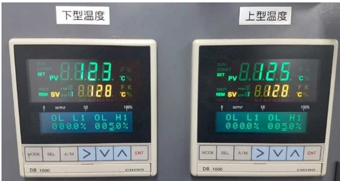
Figure 6-7: Manual adjustment of the amount of thermal energy supplied by the IR lamps; left: display for lower mold; right: display for upper mold
