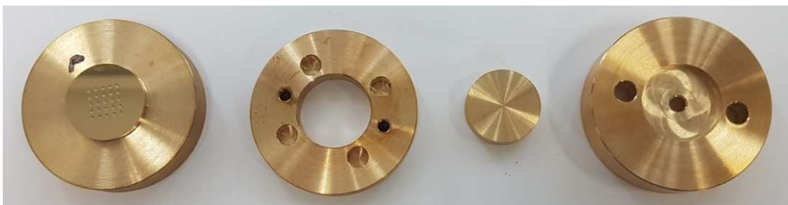
Figure 6-3: Mold parts (upper mold part already with diamond cut microlens array)
