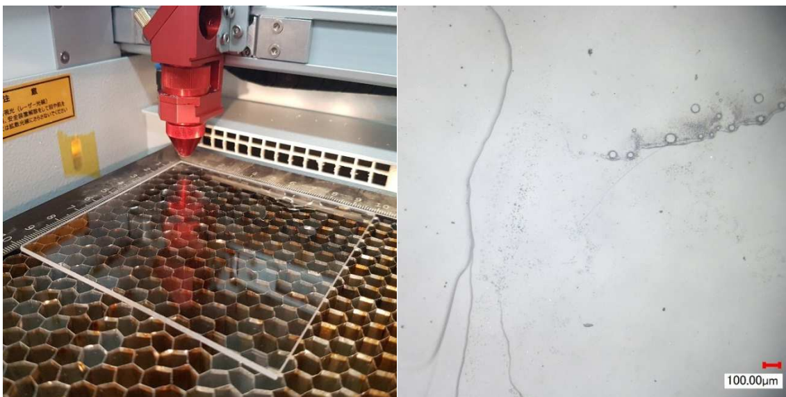
Figure 6-11: Preparation of cylindrical PMMA sheets; left: laser cutting; right: image of marks and void formation caused by heat input of the laser machine on the substrate (100x-magnification)
