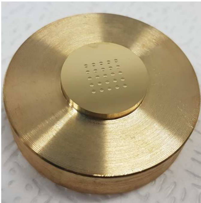
Figure 7-1: Ultra-precision machined microlens array
