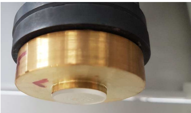
Figure 7-15: PC sample sticking to the mold after demolding
