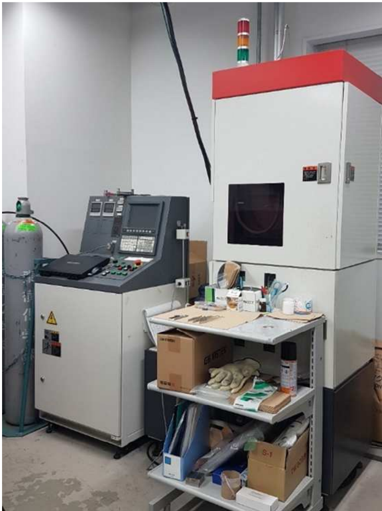
Figure 6-5: Compression molding press GMP211 (Toshiba Machine Corp., Japan)
