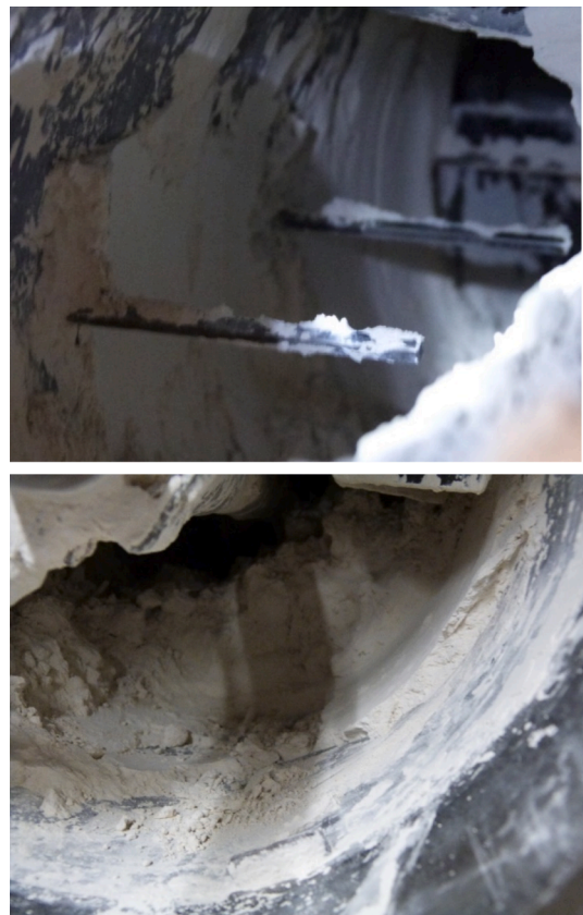
Fig. 11. Layer formation at the heat transferring wall after heating up of CaO.
