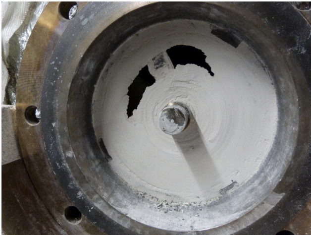
Fig. 12. Layer formation in front of the filter during dehydration.
