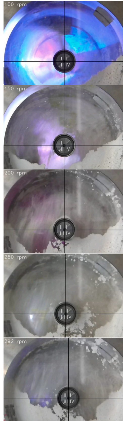
Fig. 4. Impact of the rotational speed on the bed of 0.8 \text{ kg Ca(OH)}_2 .
