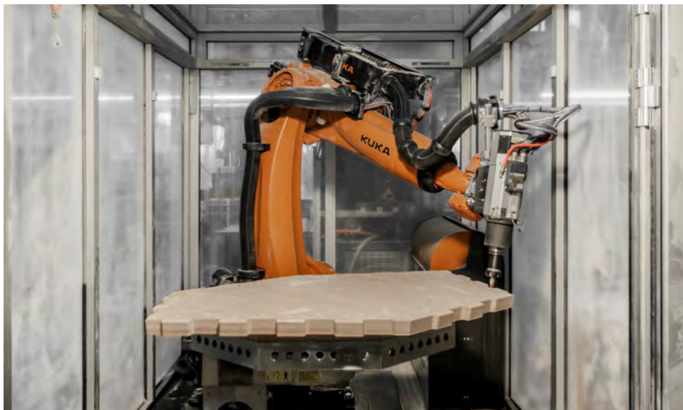
Figure 7.62: Photograph of the robot cell used in this case study and analyzed for the machinic morphospace. Its enclosure was permanent and restricted some of the parameters of the gradient building system (Image by ICD/ITKE/IIGS University of Stuttgart).
