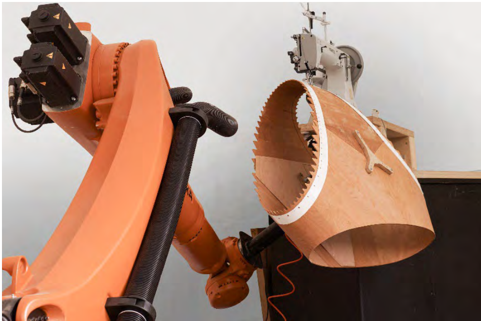
Figure 7.49: Robotic sewing of a module of the ICD/ITKE Research Pavilion 2015-16 (Image by ICD/ITKE University of Stuttgart).
