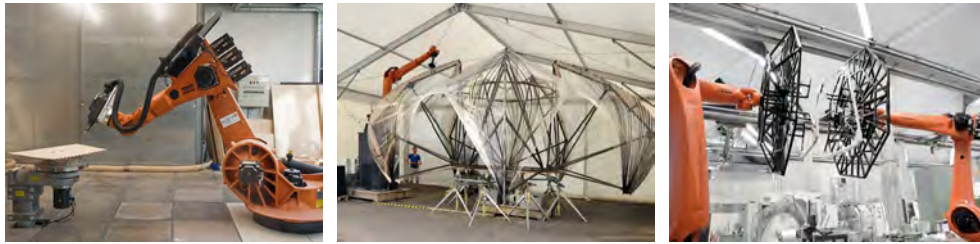
Figure 3.3: Different robotic manufacturing setups. Their work envelopes are one of many parameters that are directly related to the shapes and sizes of building elements they can produce. From left to right: manufacturing setup of the ICD/ITKE Research Pavilion 2011, the ICD/ITKE Research Pavilion 2012, and the ICD/ITKE Research Pavilion 2013—14. Images by ICD/ITKE University of Stuttgart.
