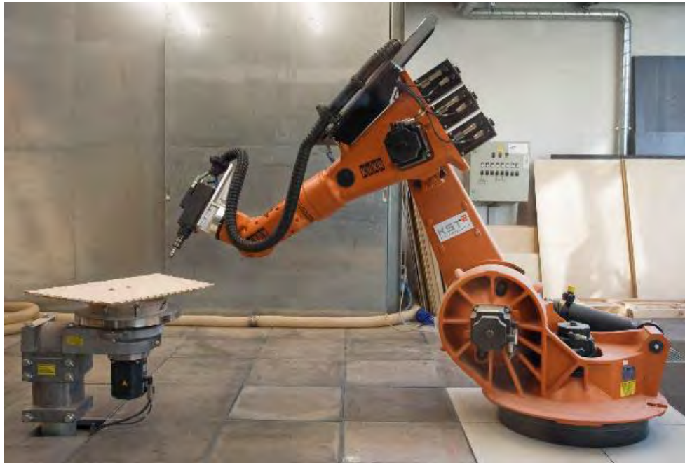
Figure 7.4: Robotic setup for milling finger joints on a turntable (Image by ICD/ITKE University of Stuttgart).
