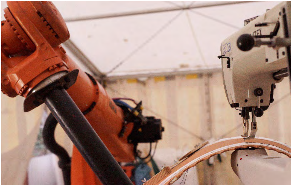
Figure 7.46: Close-up of a robot sewing process with 6mm thick plywood (Image by ICD/ITKE University of Stuttgart).
