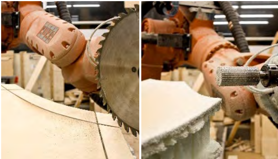
Figure 7.21: The subsequent robotic trimming process is divided into two steps. First, the outline of the cone module is trimmed using a saw blade (left), then, the foam core is cut with a foam milling bit (right) (Image by ICD University of Stuttgart).
