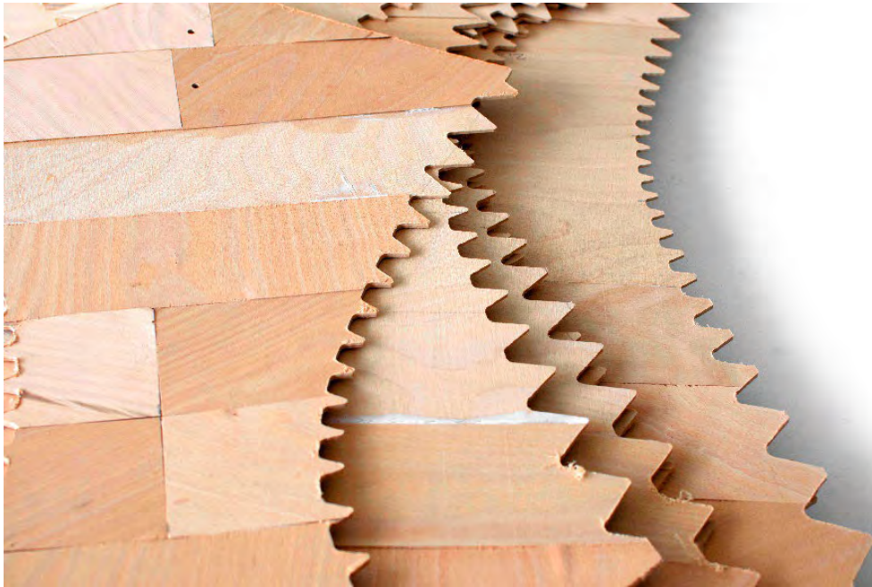
Figure 7.48: Laminated strips after CNC cutting (Image by ICD/ITKE University of Stuttgart).
