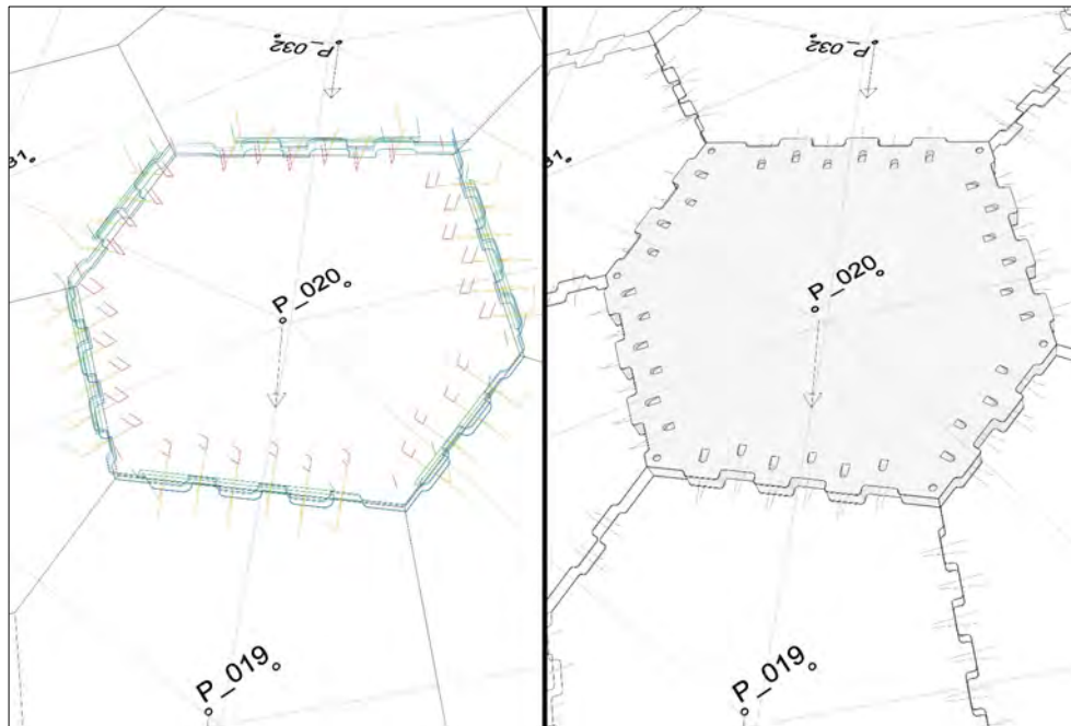
Figure 7.59: Tangent-Plane-Intersection method on double-curved surfaces results in the connection angle being equal to the angle between the normal vectors of each plate (Image by ICD/ITKE/IIGS University of Stuttgart).
