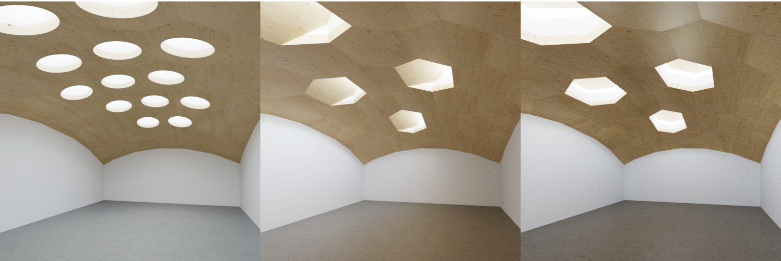
Figure 5.16: Visualization of an interior space with round prefabricated skylights (left), with rotated plates (middle), and with plates replaced by lanterns (right).
