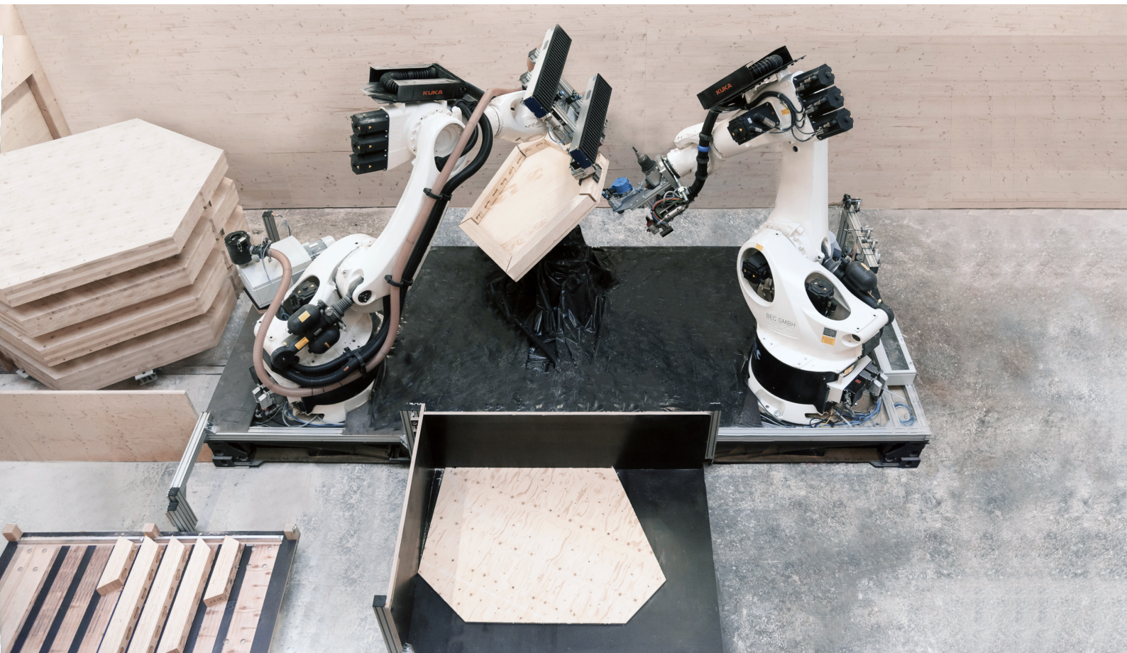
Figure A.5: Multi-robot fabrication setup for the BUGA Wood Pavilion. Image source: ICD/ITKE, University of Stuttgart
