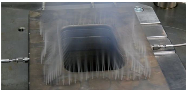
Fig. 10. Drawing die of the rectangular cup tool with free flow out of CO 2 through laser drilled microholes..
